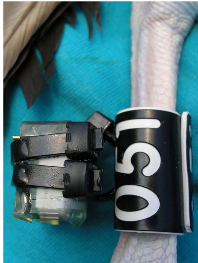
Figure 8. Example of geolocator attachment methods on a Laysan albatross.
